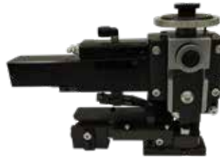
OCEAN applicator for LITEALUM terminals
