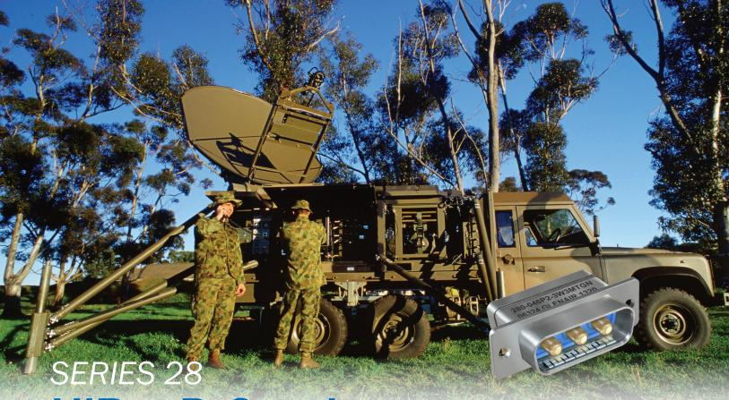
The Combo *Hi-Per*formance D-Sub connector combines size #8 power or RF contacts with size #20 signal pins. The HiPer-D® meets the need for improved performance in hostile environments. Unlike standard M24308 connectors with stamped steel shells, the HiPer-D® connector features a one-piece machined aluminum shell. The thermoset epoxy insulators are capable of 200°C continuous operating temperature. Aerospace grade fluorosilicone grommets and face seals provide environmental protection.
