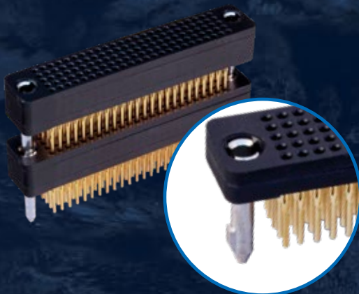
High-density (.0625" pitch) board-to-board stacking connector with solder-free press-fit (compliant pin) board mounting
