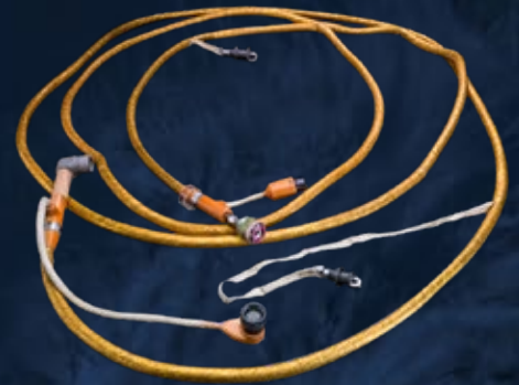
Complex space-grade cable assemblies (shown: Glenair-made "Golden Umbilical")
