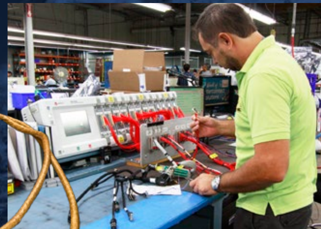
Continuity testing standard on all cable circuits
