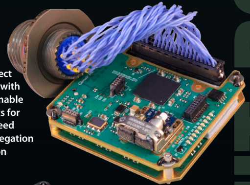
^ Small form-factor soldier-worn data hub and power distribution module with Series 80 Mighty Mouse interconnects
