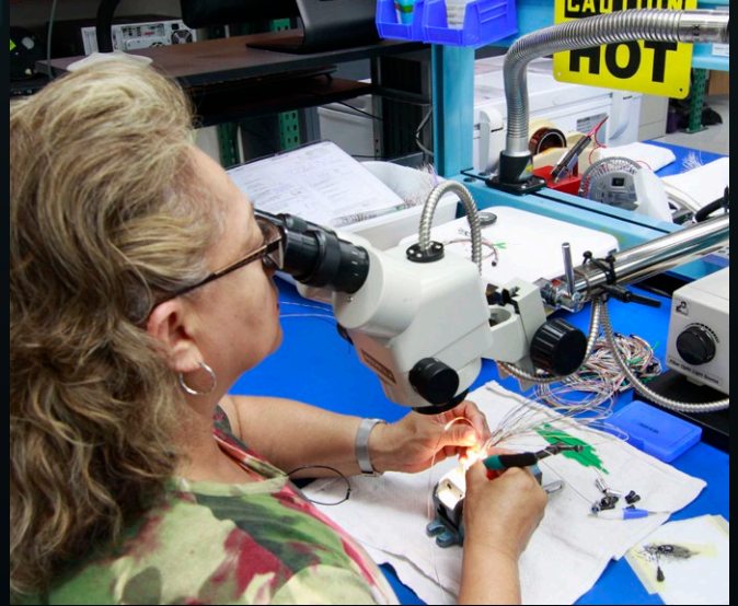
△ Small form-factor connector and cable assembly is intense, precision hand labor. Our operators have long tenure and broad experience building mission-critical point-to-point and multibranch cables.
