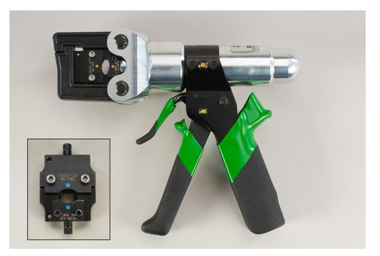
HD36 Hydraulic Crimper is a combination of a lightweight design and the precise application of 3.5 tons force to crimp power contacts too large for conventional hand tools. This tool is designed to accept the entire family of D36 dies for crimping terminals, lugs or any other special applications.
