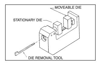
The die sets snap in and out of the crimp tool for interchangeability. A die removal tool is included with the HX23 for operator convenience.
