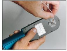
The WA22LC-X1 tool features a smaller profile and lighter weight which makes it especially useful for second end terminations on vertical and horizontal wiring form boards. Most size 20 and smaller contacts can be terminated with this tool.
